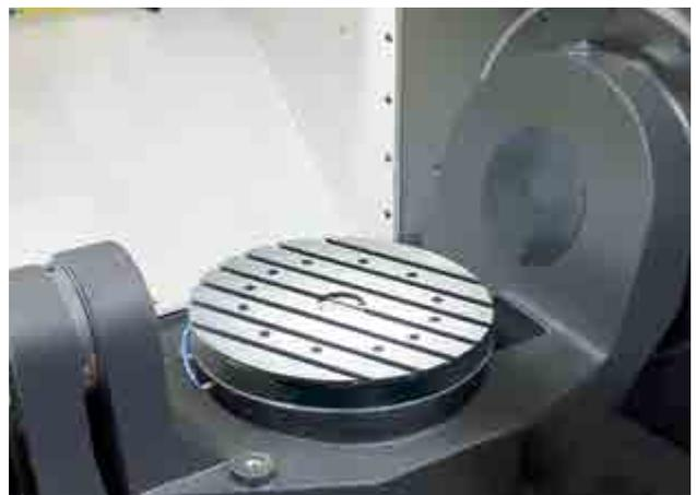
Rotary swiveling table with parallel grooves
