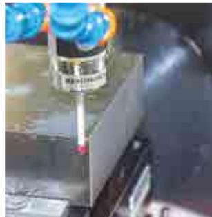
Infrared measuring probe
