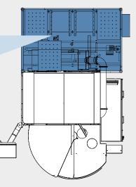
Mikron MILL X 600 / 800: linear-type magazine
