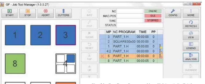
User friendly software for one machine with integrated pallet changer. Assign NC programs to pallet position by drag and drop on a touch screen, close to the pallet changer.
