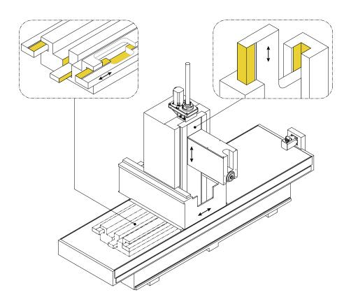
The whole quality of the MÄGERLE Grinding Centers is based on the unique design principle. The axis structure is supported by hydrostatic wrap-around guideways on a thin oil film and is completely separated from the machine bed. As a result MÄGERLE grinding machines can withstand high loads without signs of wear — even in long-term use. The oil film has a vibration-damping effect and guarantees high-precision machining of simple or complex workpieces.
