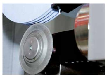
The dressing of the grinding wheels is a crucial factor for the efficiency of the grinding process. With overhead and table dressing devices, MÄGERLE provides professional solutions for the various requirements of this process step. The potential of the overhead principle is developed in continuous dressing (CD) and inprocess dressing (IPD). Table dressing devices are used
