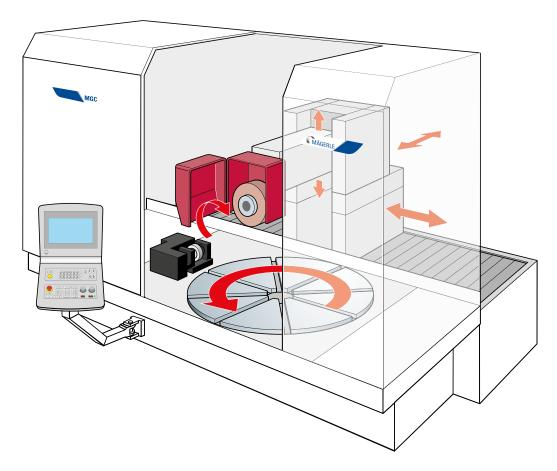
With table diameters of up to 2.5 meters and a maximum load bearing capacity of 12 tons, the MGC RH grinding center is unequalled throughout the world. Well-known companies in the turbine industry rely on this powerful concept. This grinding center is unrivalled particularly when it comes to
