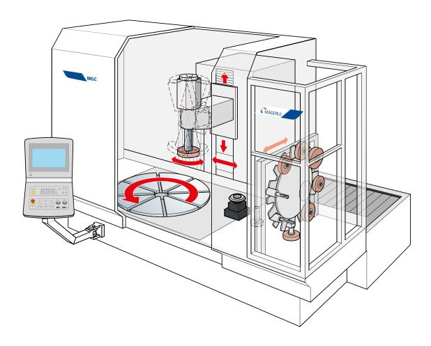
Versatility with the highest production quality level is the outstanding strength of this vertical grinding machine. It demonstrates its capabilities particularly in the manufacture of bearing rings, where optimum runout characteristics are required for maximum smooth running. Equipped with rotary table and fully automatic tool changer, this vertical grinding machine can master other functions in addition to grinding. Whether turning,
