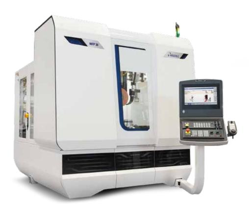
The compact MFP 30 5-axis grinding center from MÄGERLE is ideally suited for grinding complex geometries, particularly those of blades and vanes or heat shields for aviation turbines. The workpieces to be machined are ergonomically loaded into the work area directly from the front. Heavy workpieces with a clamping fixture can be loaded from the top using a crane. The compact and space-saving design allows optimal use of the available production area and enables an effective production flow.
