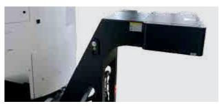
To increase the tank capacity, an external filter system with a capacity of 650l is available.
