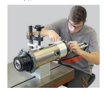
Included in delivery is the smart machine module Advanced Processing System (APS) for the reliable recording and display of vibrations during the Milling process.
