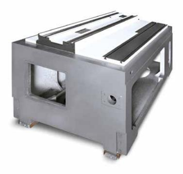
The machine bed, comprising of gray cast iron, is cast from a single piece and forms the base for mounting the high-precision cross slide table and the grinding spindle mounting block. The support of the guides for the X axis is cast directly into the machine base. The remaining area on the upper part of the machine base conveys the coolant around the base back into the coolant unit or the coolant cleaning unit, via a coolant tank.
