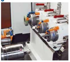
The modular grinding spindle support concept enables optimal adaptation to the respective grinding task. The grinding spindle supports comprise of permantly boltedon solid mounting blocks, either in a single or twin version, depending on the requirements. One, two or three spindles in a linear arrangement can be used in the basic configuration. The use of up to three spindles is possible depending on the specific geometrical situation. In the case of two or three grinding spindles the maximum
