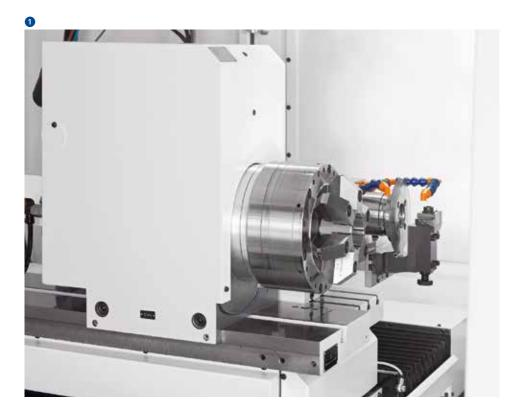
The high-precision workhead is equipped with special bearings and guarantees the highest roundness accuracy. The spindle nose complies to the DIN/ISO 702-1 standard.
