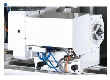
With its high-precision roller bearings the workhead is used for grinding between fixed centres and for live spindle grinding. The powerful workhead spindle has a MT4 or ISO50 fitting taper.
