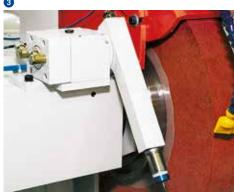
The turret wheelhead can be used for both external and internal grinding; it can be equipped with an external grinding wheel (right) and an internal grinding spindle for this purpose. With extreme precision, the user can manually (2.5°) index the turret wheelhead in a Hirth gear within a swiveling range of -15°/+195°.
